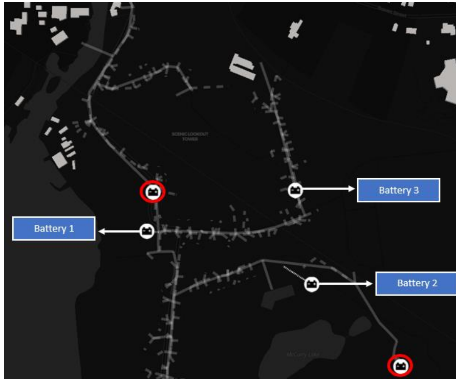
Figure 7. Location of 3 x 750 kW Batteries
