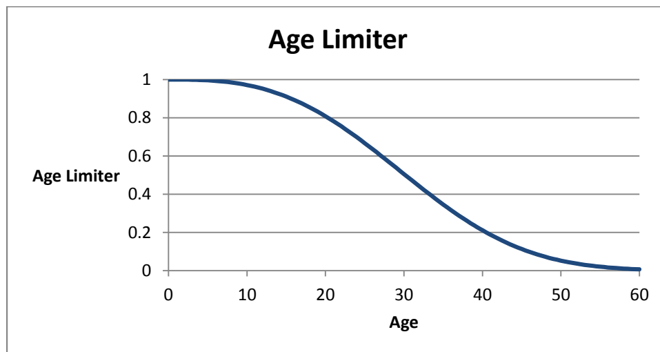
Figure A 2-1 Pad Mounted Transformers Age Limiter
