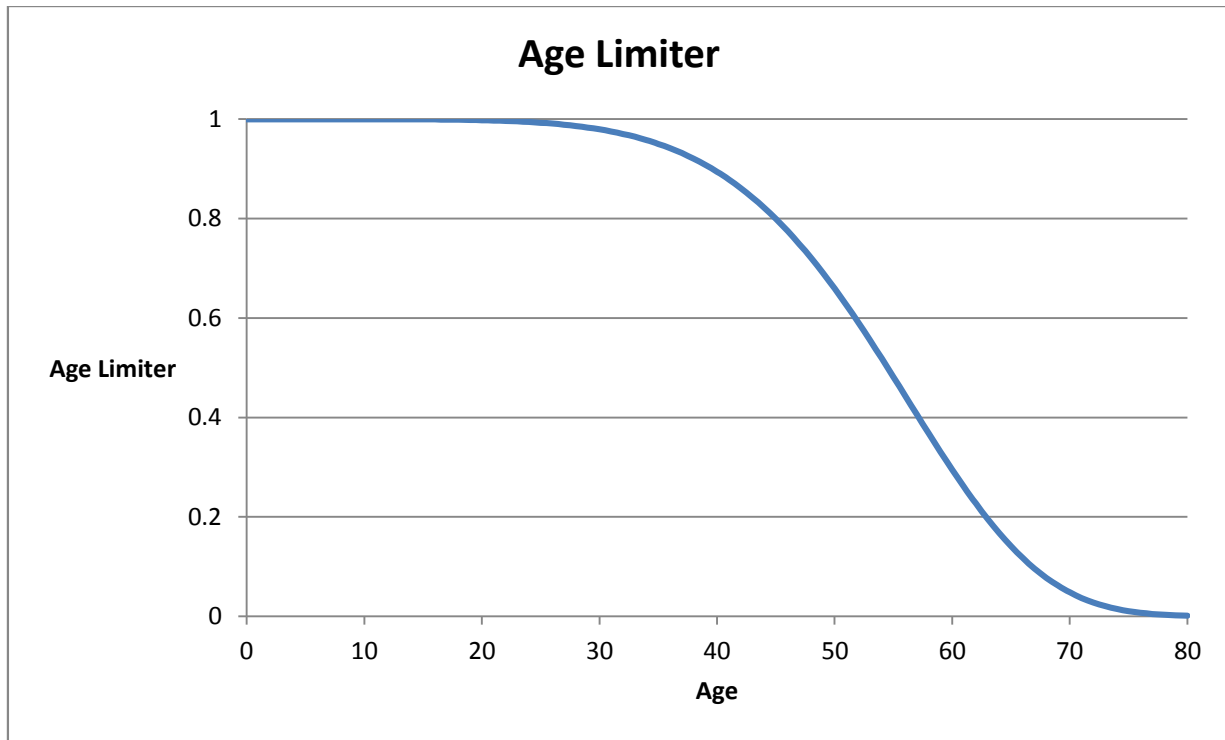
Figure A 1-1 Station Transformers Age Limiter
