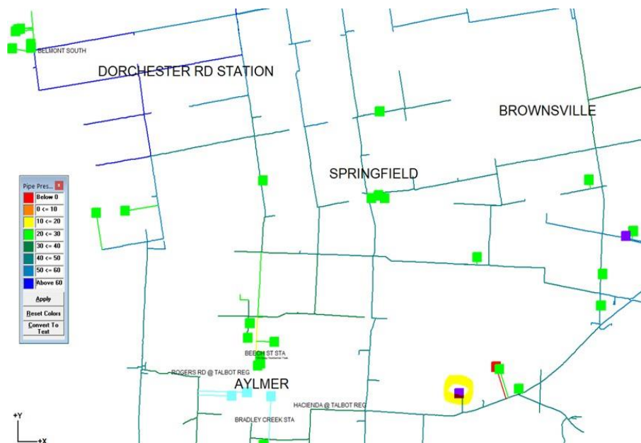
Fig 13. New 4” Pipeline on Wilson Road, January 2028 loading case without 9608 Carter Road proposed client
