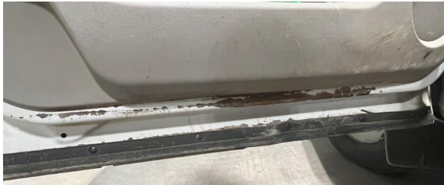
Figure 5: Vehicle 14 interior rust
