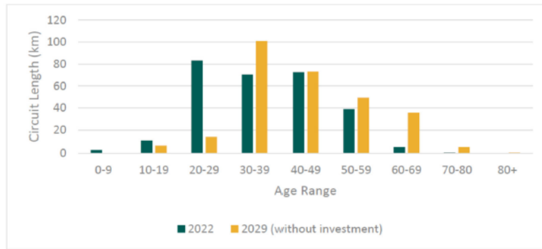
Figure 9: Age Demographics of Direct-Buried (“DB”) Cable XLPE in Underground Horseshoe System as of 2022 and by 2029 (without Investment)
