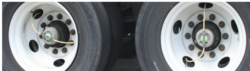
Figure 24: Automatic Tire Inflation System (courtesy NACFE)
