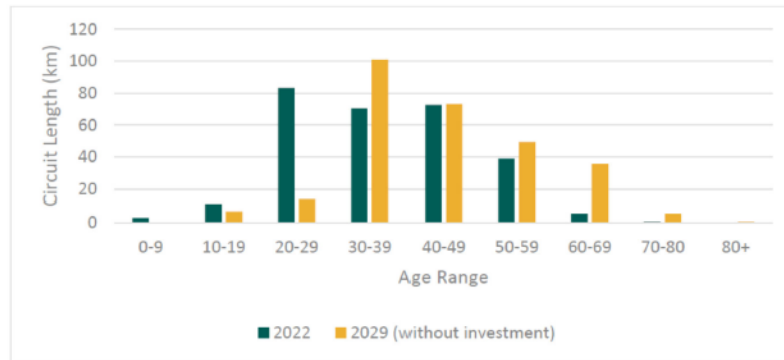
Figure 9: Age Demographics of Direct-Buried (“DB”) Cable XLPE in Underground Horseshoe System as of 2022 and by 2029 (without Investment)
