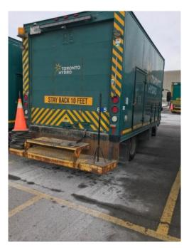
Figure 2: Corrosion on Cube Van Steps
