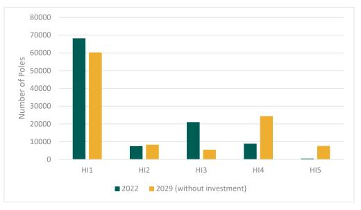
Figure 18: Condition of Wood Poles in 2022 and 2029 (without investment)
