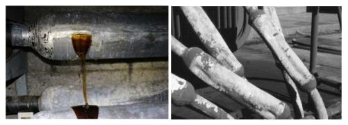
12 Figure 4: Sample PILC Joint with a Split Sleeve, i.e. Leaker (Left) and Collapsed Cable Splice (Right)
