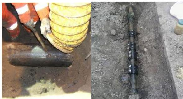
Figure 5.2-7: Bare and unprotected steel failures
