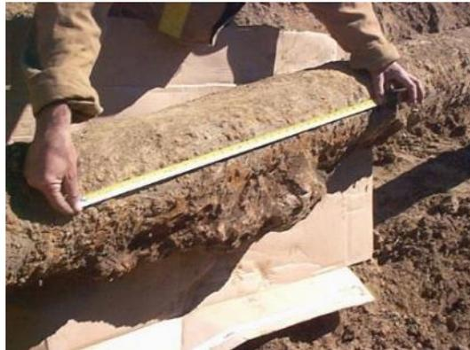
**Figure 5.2-55: Corrosion**
