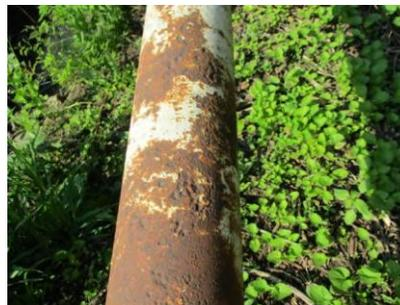
**Figure 5.2-14: Coating degradation and corrosion pitting**
