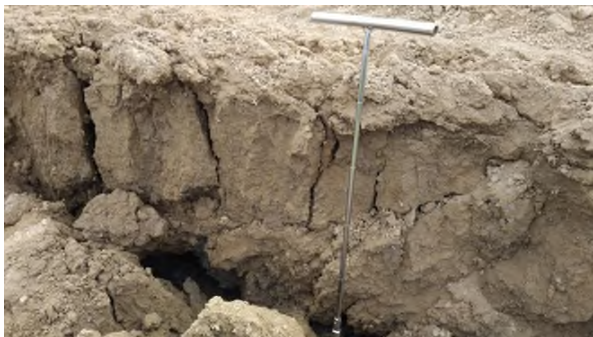
Sept 19 - P107 breakage of subsoil into columnar structure indicative of good installation conditions
