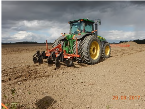
e) Sept 29 - P121 paratyl plow decompacting topsoil to 30cm depth
