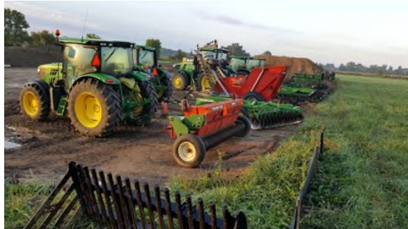
September 19 - HM44 farm equipment used for soil decompaction and restoration
