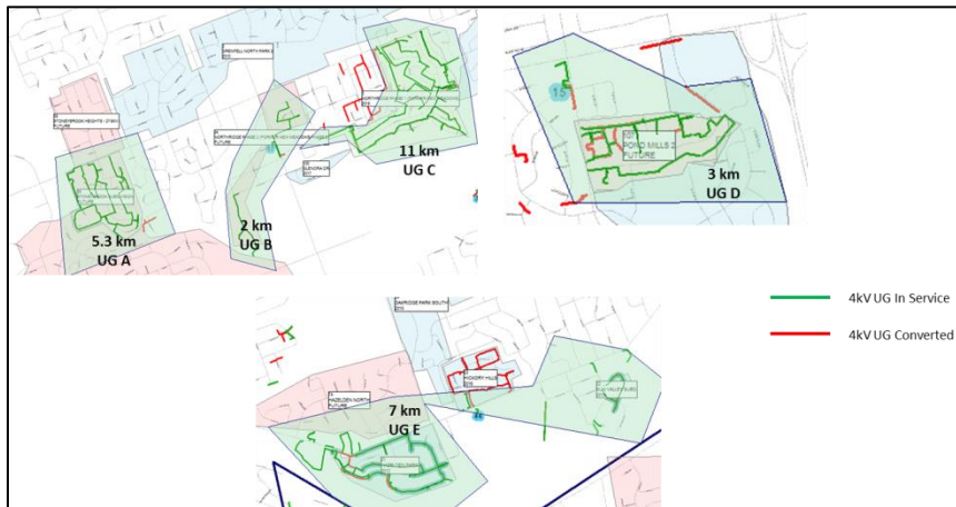
Figure 15: Most Significant 4.16kV Underground Areas Remaining
