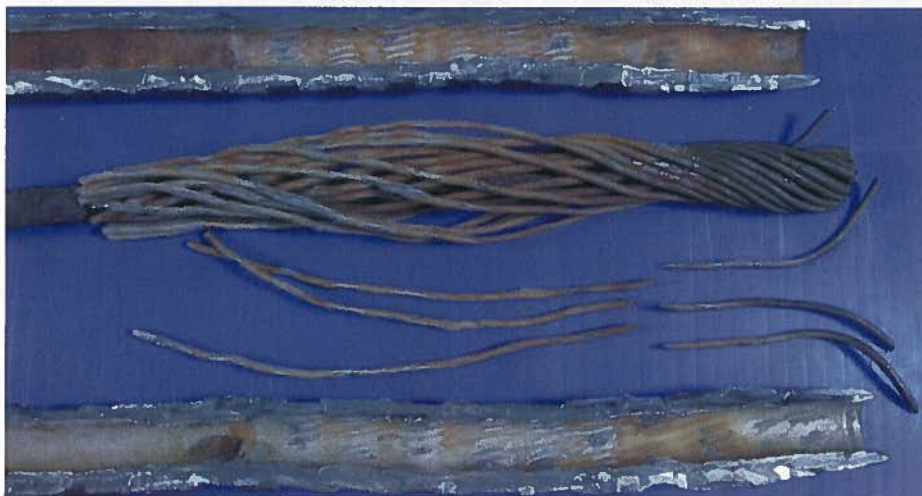
Figure 3b - Non-Failed Side - Three Broken Aluminum Wires Inside Splice
