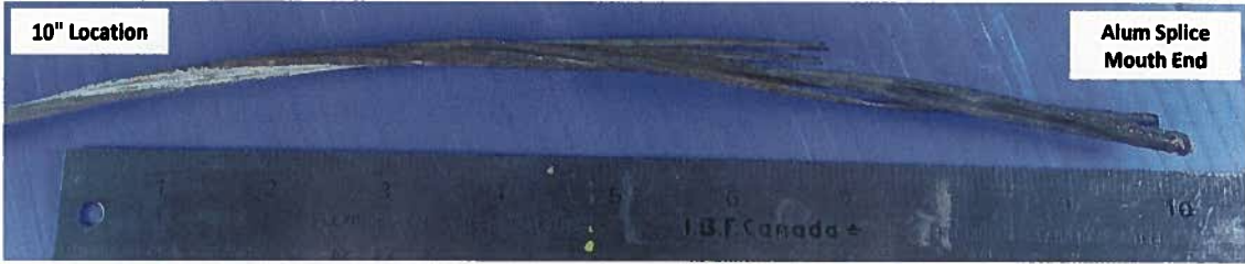
Figure 12a - Failed Side - Moderate to Heavy Rusted Wires (for about 10 inch length)
