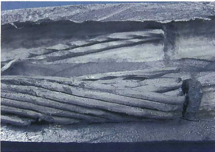
Figure 5: Failed Connector: solid stop in place
