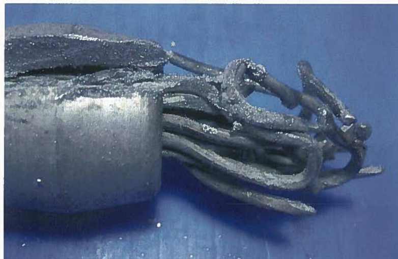
Figure 2: Failed Connector End: note conductor strands melting
