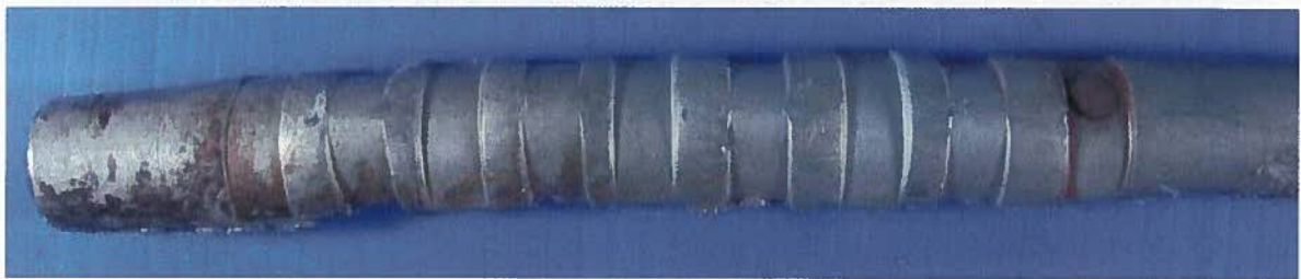
Figure 1a - Failed Side Crimp Locations
