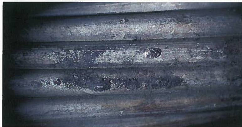
Figure 2c - Outer Surface - Darker Contaminated Side - Close-up of Melted Spot
