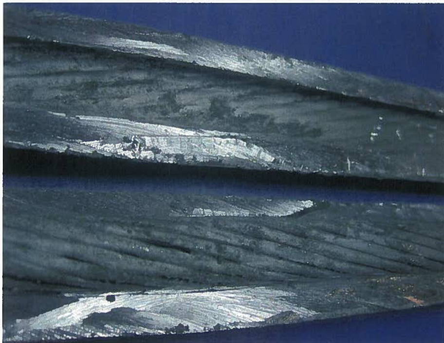
Figure 13: Dissected Connector: conductor is clean, no corrosion, no visible contamination
