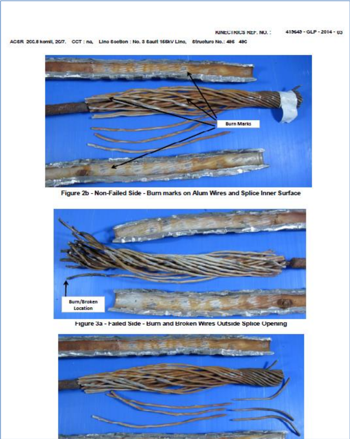
Figure 5 – Deteriorated Conductor Examined in the Kinectrics Study
