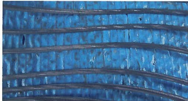
Figure 4b - Outer Layer Wires - Inner Surface - Close-up
