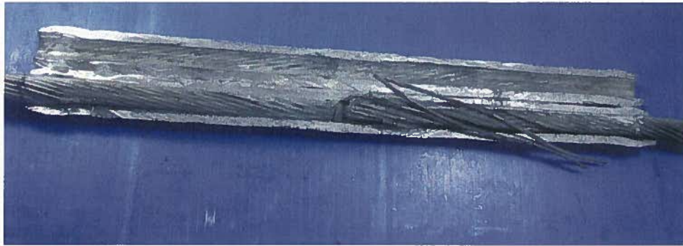
Figure 20: Dissected Connector: opened to review inner condition; note some strands moved during dissection
