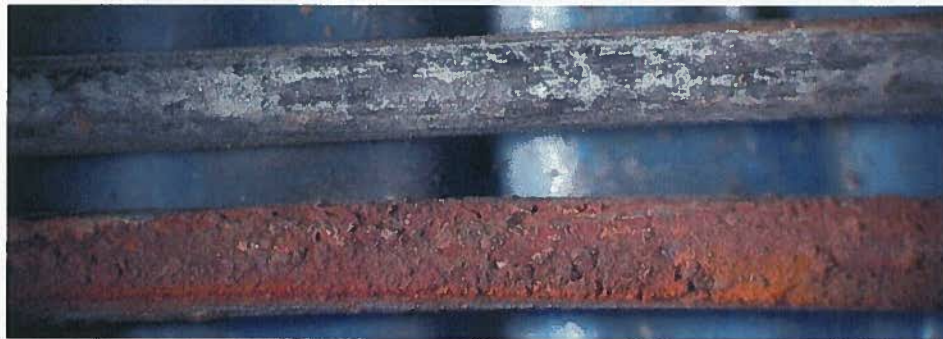
Figure 8c - Steel Wires - Inner Surface (top) & Outer Surface (bottom)
