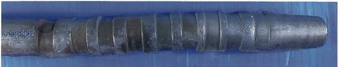
Figure 1b - Non-Failed Side Crimp Locations
