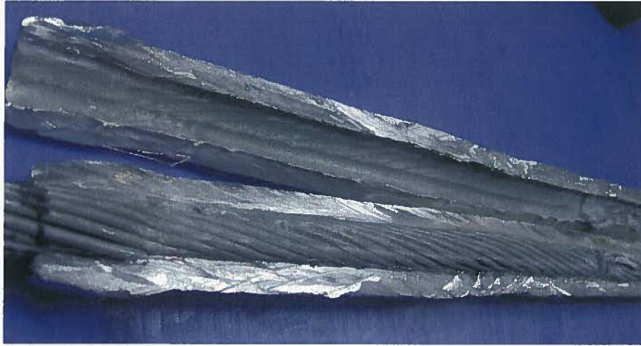
Figure 17: Dissected Connector: proper conductor location, no signs of corrosion
