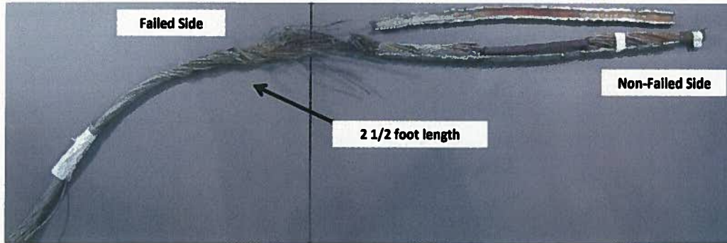
Figure 9 - Failed Side - 2 1/2 foot Sample
