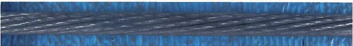
Figure 5a - Inner Layer - Outer Surface - Darker Contaminated Side
