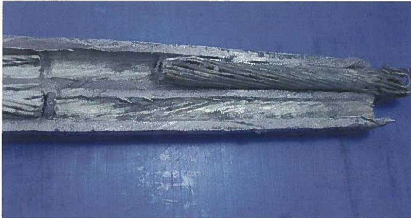
Figure 6: Failed Connector: dislodged conductor on failed side
