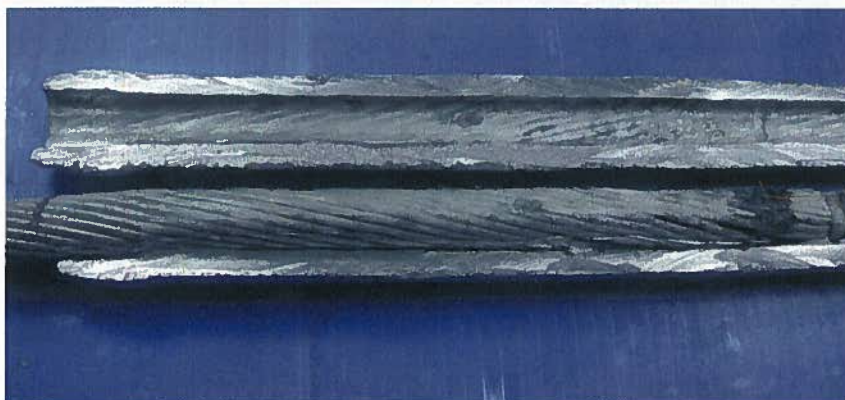
Figure 11: Dissected Connector: proper conductor positioning, no corrosion
