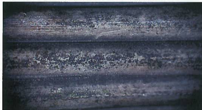
Figure 2b - Outer Surface - Darker Contaminated Side - Close-up
