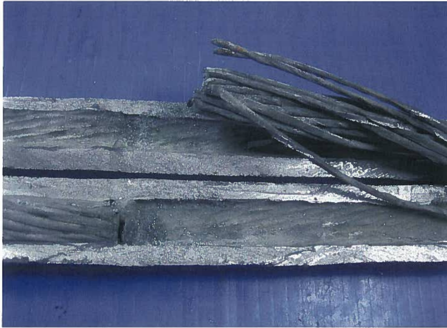
Figure 22: Dissected Connector: conductor on right-hand side removed to show connector sleeve; note black residue on the conductor surface in this area
