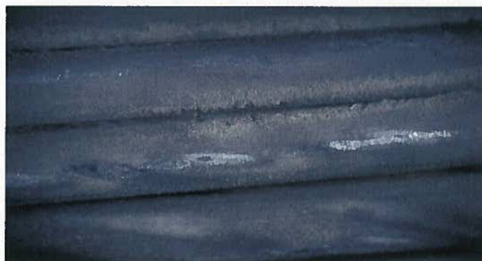
Figure 5b - Inner Layer - Outer Surface - Darker Contaminated Side - Close-up
