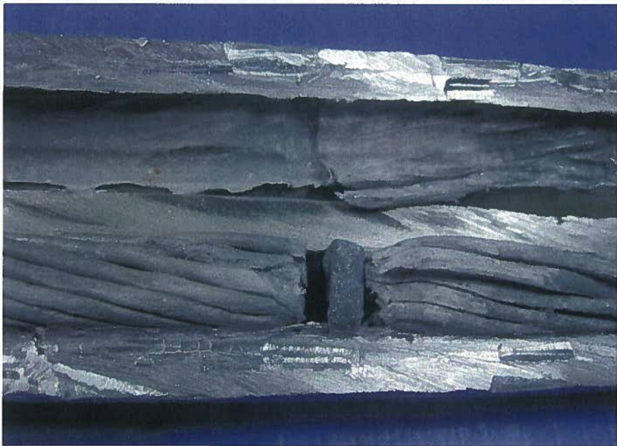
Figure 18: Dissected Connector: solid stop located, conductor on both sides properly positioned
