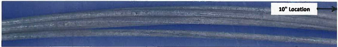
Figure 12b - Failed Side - Wires Beyond 10 Inch Location, No Corrosion
