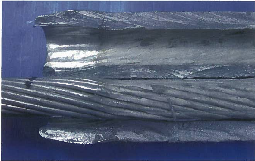
Figure 4: Failed Connector: non-failed side, clean contact areas, no corrosion
