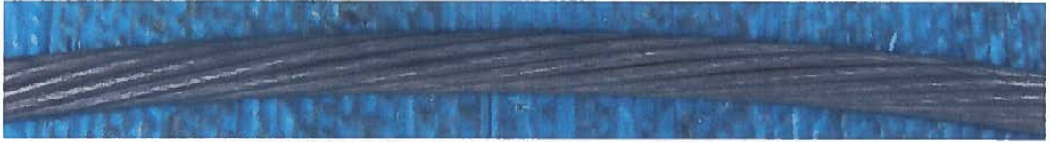
Figure 6a - Inner Layer - Outer Surface - Lighter Contaminated Side
