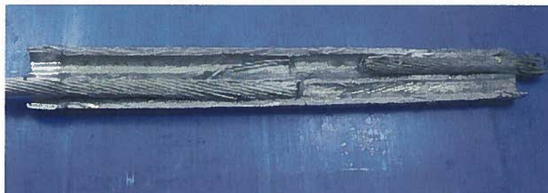
Figure 3: Failed Connector: opened to review inner condition
