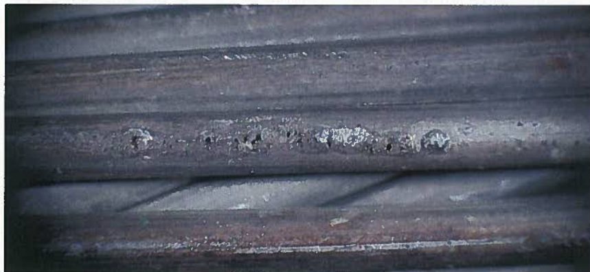
Figure 3d - Outer Surface - Grey Side - Close-up of Melted Spot
