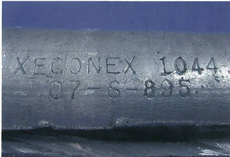
Figure 15: Connector Dissected: note manufacturer's P/N, date code (same P/N on all reviewed connectors)
