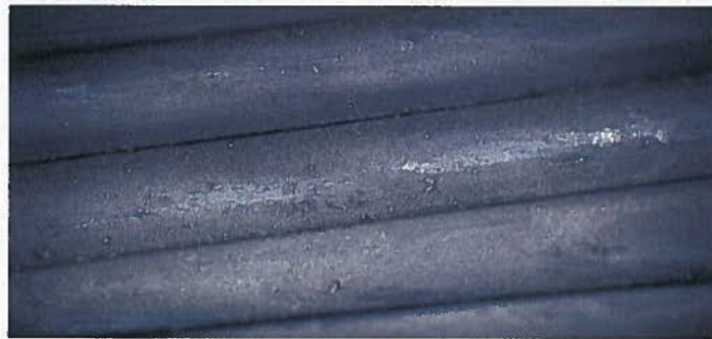
Figure 6b - Inner Layer - Outer Surface - Lighter Contaminated Side - Close-up
