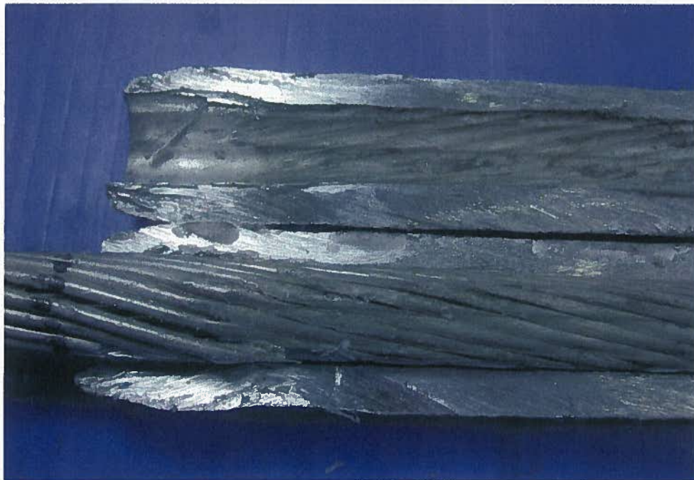
Figure 21: Dissected Connector: clean contacts, no corrosion
