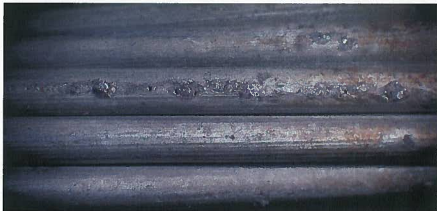
Figure 3c - Outer Surface - Grey Side - Close-up of Melted Spot
