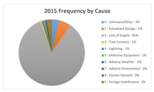
The 2014 and 2015 Figures demonstrate that the majority of outages resulted from Loss of Supply from HONI. This, for the most part, is due to scheduled outages performed by Hydro One to complete maintenance and upgrades to the transmission line into Sioux Lookout which is a radial feed. In 2014, SLHI had 10,258 service interruptions to customers; 8,203 of these interruptions were due to Loss of Supply. Service in 2015 saw 6,586 customer interruptions, and 5,581 of them were from Loss of Supply.
