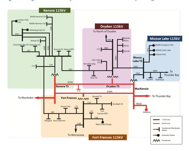
The regional 115 kV sub-systems (as shown in Figure 4-4) enable power to be delivered to communities and customers in the West of Thunder Bay Sub-region. There are four 115 kV sub-systems in the sub-region:
