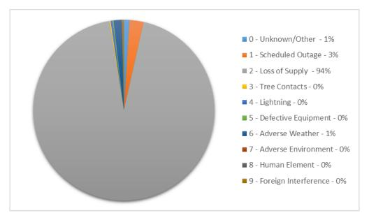
Loss of Supply is responsible for the majority of the outage hours to customers in 2014 and 2015. In 2014, the total customer interruption hours totaled 17,170, of which 13,624 were due to Loss of Supply. In 2015, SLHI customers experienced 31,254 interruption hours, which is a significant increase, yet Loss of Supply from HONI was responsible for 29,356 (94%) of those hours.
