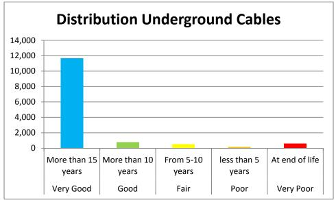
The majority of the underground primary cables have been installed since 1990, and as such are considered to be in very good condition based on age. Approximately 4% of the cables in the Sioux Lookout Hydro system are currently beyond their expected useful life and are represented by only three older installations. About 5% of the asset will reach its expected life span within the next 5-10 years, and are represented by only three installations.
