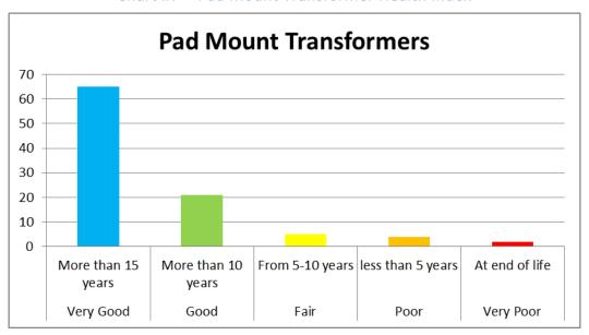
Since the majority of SLHI's underground infrastructure is relatively new, most of the pad mounted transformers were assessed to be in excellent condition.
