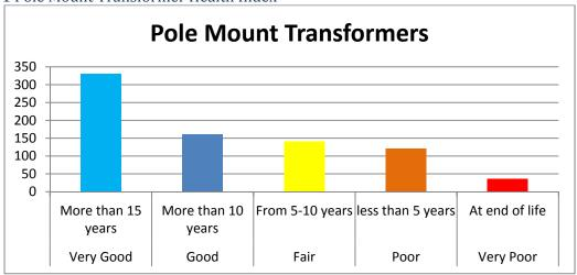
The pole mount transformers classified as being in "very poor" condition are ones that are listed in the database as being 40+ years of age or those that have no age listed in the database.
