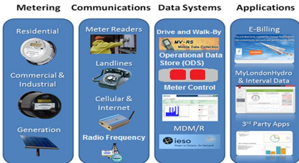
8 Figure 2-5 – Scope of Metering Services
