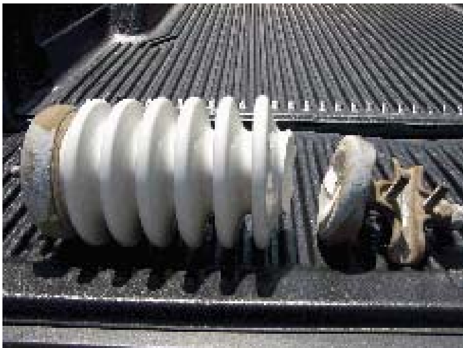
1 Figure E: Broken Porcelain Insulator
