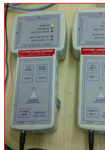
Figure 1, Example Hand-Held Meter Initialization Tools
