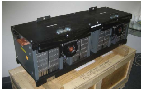
Altairnano Super Module 6.4 kWh (Nominal 18.4 V 2800 Ah)
