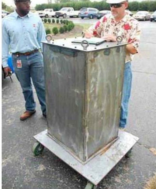
Figure H-3. Lowering 25 kWh Battery Container into Subterranean Vault
