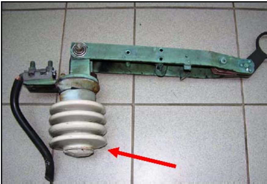
1 Figure 47: Broken Porcelain In-Line Switch
