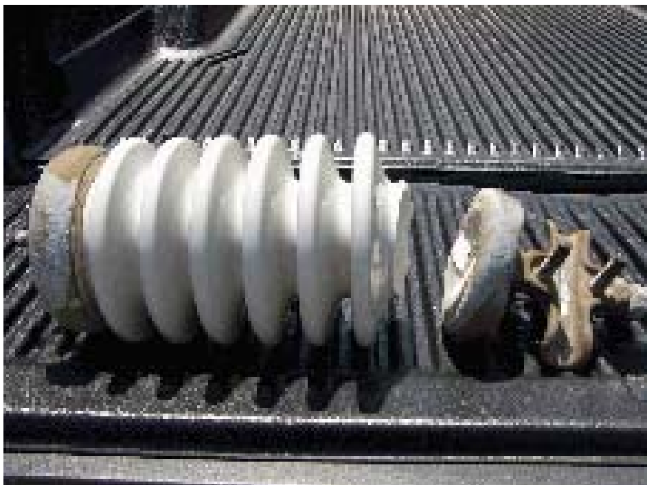
4 Figure 55: Broken Porcelain Insulator
