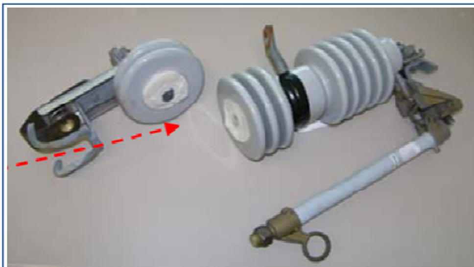
7 Figure 39: Broken Porcelain Switch Returned From Field
