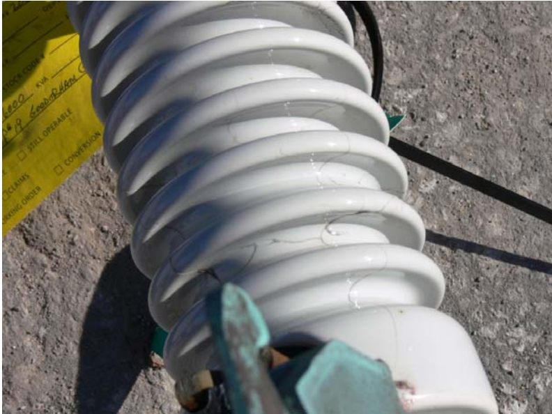
2 Figure 42: Failed Porcelain SMD-20 Switches from OS 46849 P19 Gooderham at Brian Ave
