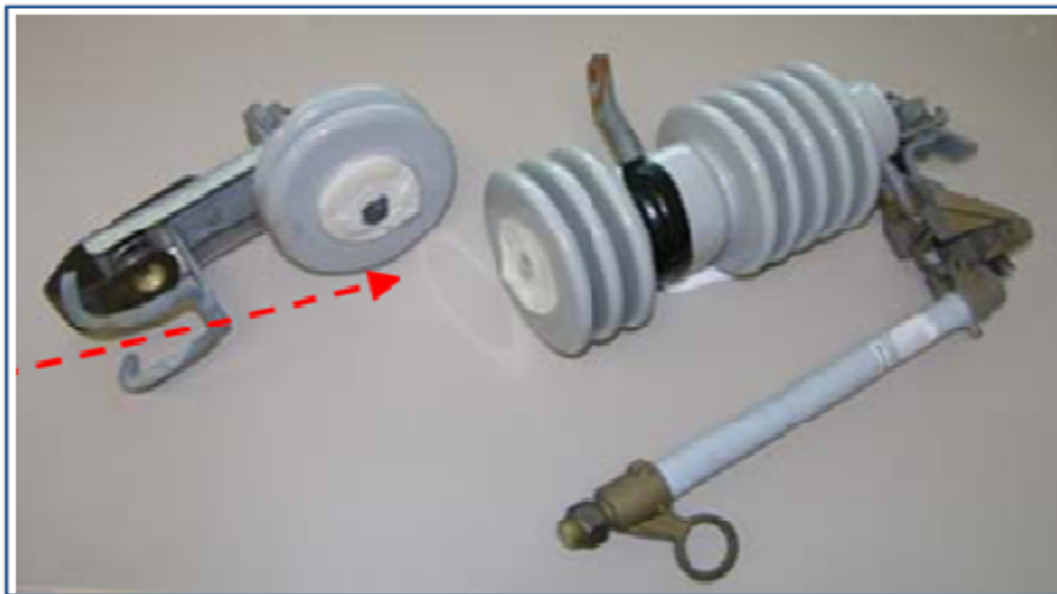
12 Figure D: Broken Porcelain Switch Returned From Field
