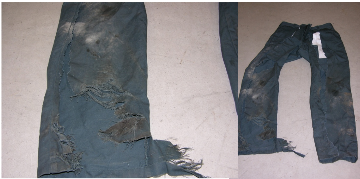
9 Figure 10: Burn marks and tears after worker experienced an arc flash from a cable that 10 required piecing out (April 27, 2007)
