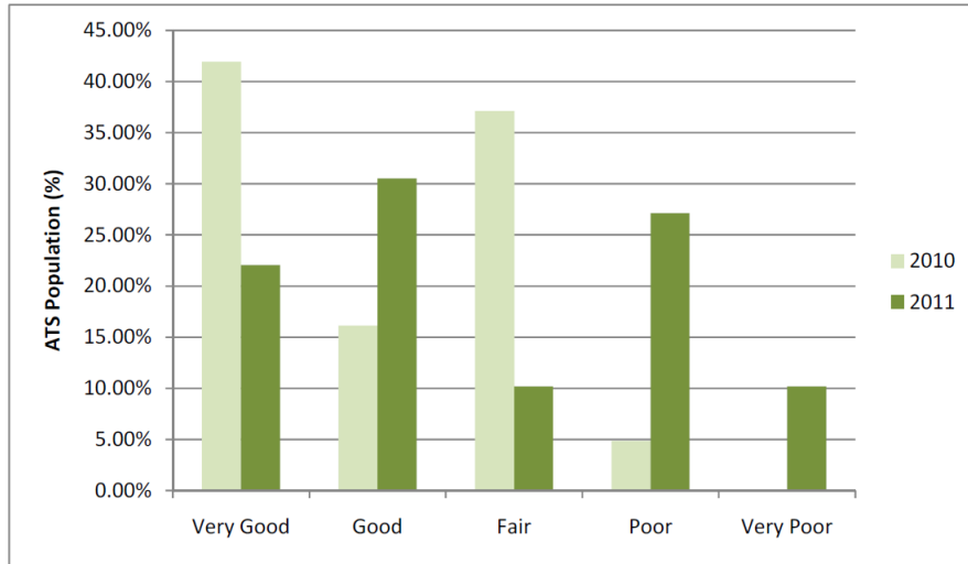
Figure 2: Asset Condition for ATS units
