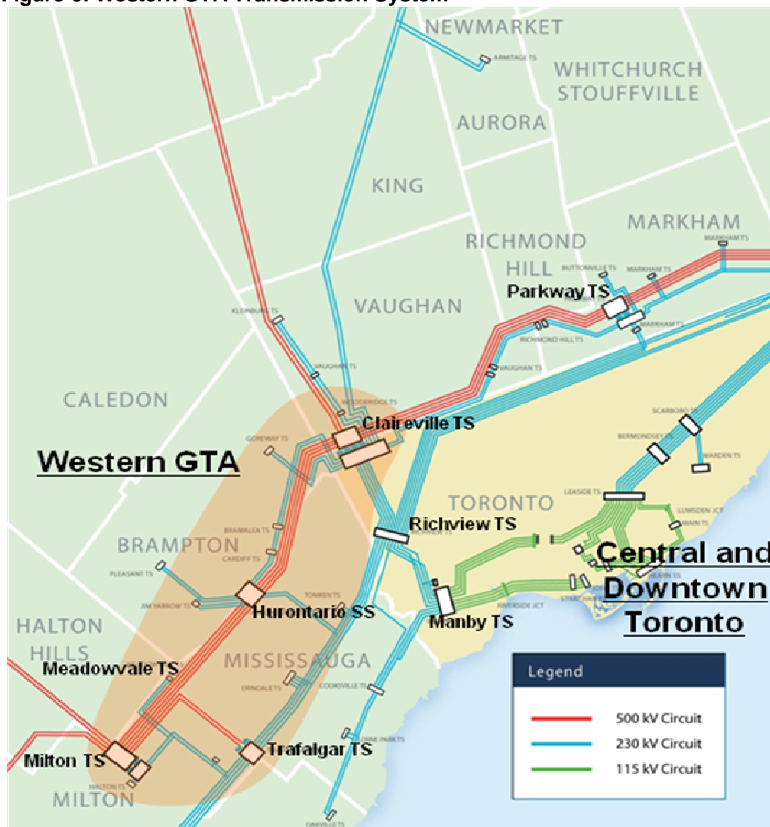
Figure 6: Western GTA Transmission System
